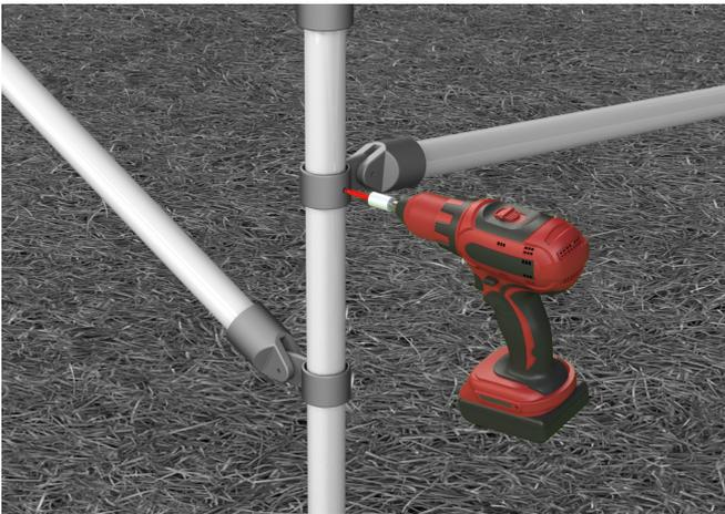
With all Hollander fittings properly torqued, locate the Tie Brace's #17 ADJ. ELBOW's. On the opposite side of the set screw, drill a pilot hole using a #3 Drill bit.
