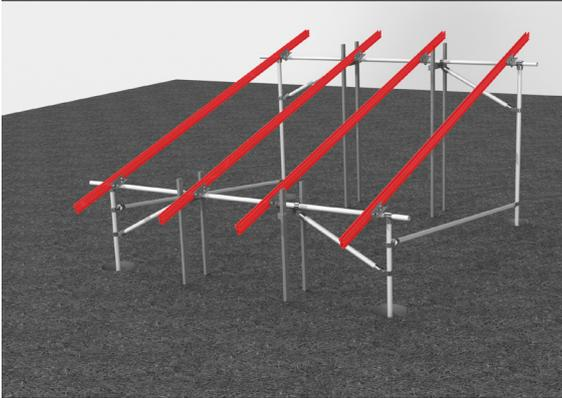
Set CrossRail 80 on to horizontal galvanized pipe at spacing required to support PV modules per the panels' manufacturer guidelines.
